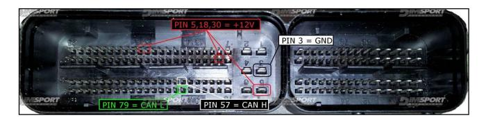
To the power feeding pins 5,18,30 (+12V) you can connect both wires red (VECU) and orange (VKEY) of the F32GN037C cable, they both have 12V signal.
