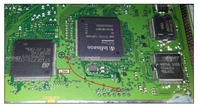
A different solution is to connect the BOOT wire directly to the orange BOOT clamp on the F34DM011 adapter. Check that the yellow BOOT jumper is set in ON position. Connect then the flat cable to the Trasdata.
