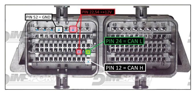
**WARNING:** in order to read&write properly the ECU it is necessary to perform two LINK, remove them before placing back the ECU into the vehicle.
