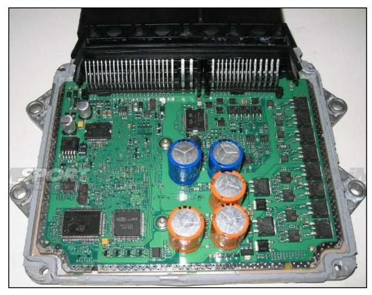
To enable the reading/writing procedure it is necessary to remove the resistor 0 shown in the following picture. After the modification it is NOT necessary to solder it back.
