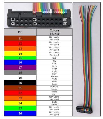
WARNING: connect the wirings without any shortcircuits between the pads
