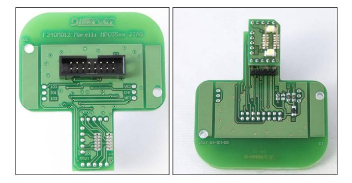
Place the F34DM012 adapter as shown in the following pictures, check the correct position on the del PIN 1.
