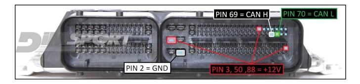
To the power feeding pins 3,50,88 (+12V) you can connect both wires red (VECU) and orange VKEY) of the F32GN037C/D cable, they both have 12V signal.
