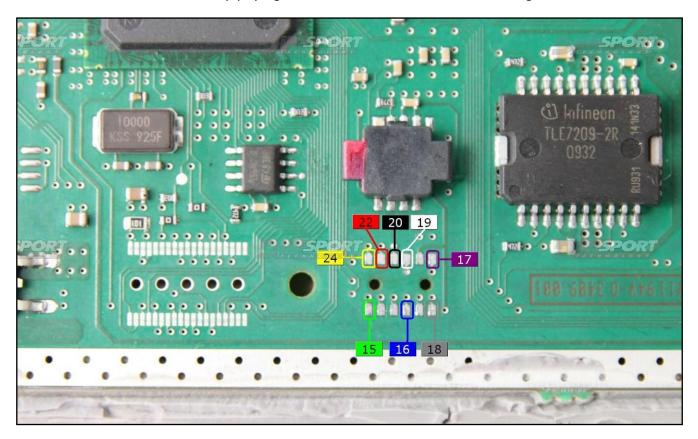
**WARNING**: solder the wires by paying attention NOT to short-circuit the signals of the wires
