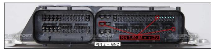
To the pin 3,50,88 you can connect both wires red and orange, they both have 12 Volt signal.
