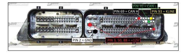
To the power feeding pins 3,50,88 (+12V) you can connect both wires red (VECU) and orange VKEY) of the F32GN037C-D cable, they both have 12V signal
