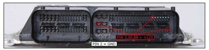
To the pin 3,50,88 you can connect both wires red and orange, they both have 12 Volt signal.
