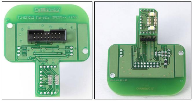
Place the F34DM012 adapter as shown in the following picture, check the correct position of the PIN 1  $\,$
