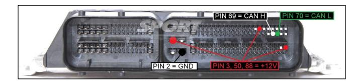
To the power feeding pins 3,50,88 ( $\pm$ 12V) you can connect both wires red (VECU) and orange VKEY) of the F32GN037C-D cable, they both have 12V signal.
