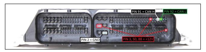
To the power feeding pins 3,50,88 (+12V) you can connect both wires red (VECU) and orange VKEY) of the F32GN037C cable, they both have 12V signal.
