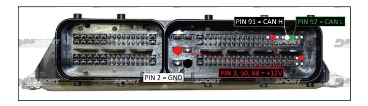
To the power feeding pins 3,50,88 ( $\pm$ 12V) you can connect both wires red (VECU) and orange VKEY) of the F32GN037C-D cable, they both have 12V signal.
