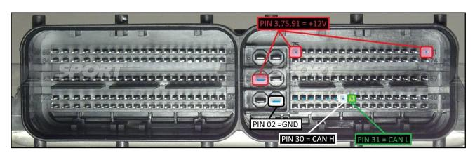
To the power feeding pins 3,75,91 (+12V) you can connect both wires red (VECU) and orange VKEY) of the F32GN037C cable, they both have 12V signal.
