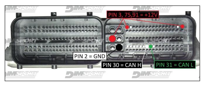
To the power feeding pins 3,75,91 (+12V) you can connect both wires red (VECU) and orange VKEY) of the F32GN037C/D cable, they both have 12V signal.
