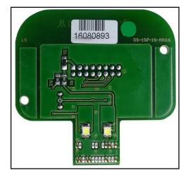
JTAG pads for the communication are placed below the microprocessor, for this connection the bridges (LINK) shown at pg. 6 are required. Check the PIN 1 position for a correct orientation of the adapter F34DM025.
