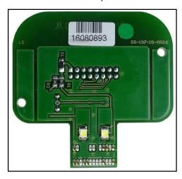
JTAG pads for the communication are placed below the microprocessor, for this connection the bridges (LINK) shown at pg. 6 are required. Check the PIN 1 position for a correct orientation of the adapter F34DM025.
