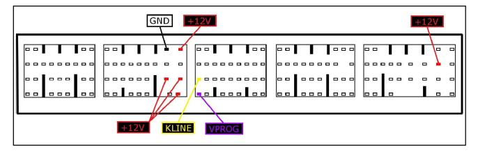
To the power feeding pins +12V you can connect both wires red (VECU) and orange (VKEY) of the F32GN037C cable, they both have 12V signal.
