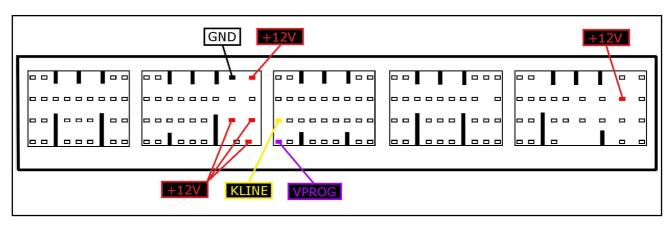
To the 5 power feeding pins you can connect both wires red and orange, they both have 12 Volt signal.
