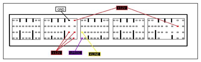
To the 5 power feeding pins you can connect both wires red and orange, they both have 12 Volt signal.
