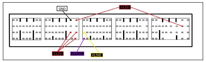
To the 5 power feeding pins you can connect both wires red and orange, they both have 12 Volt signal.
