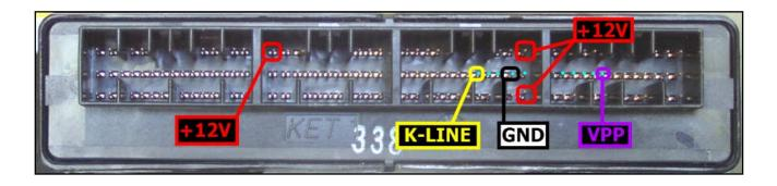
To the 3 power feeding pins you can connect both wires red and orange, they both have 12 Volt signal.
