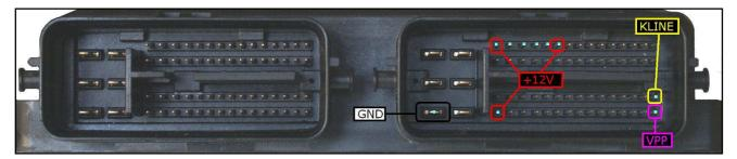
To the 3 power feeding pins you can connect both wires red and orange, they both have 12 Volt signal.
