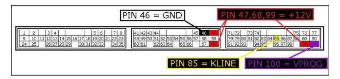
To the 3 power12V pins you can connect both wires red and orange, they both have 12 Volt signal.
