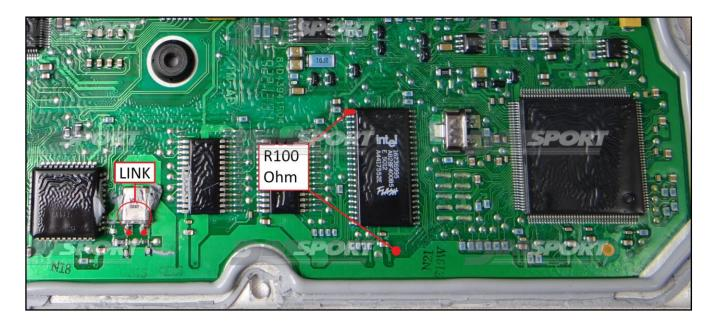
All these connections must be removed before restoring the ECU into the vehicle.
