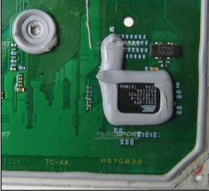
In order to perform the BDM reading it is necessary to make a little bridge on the quartz as shown in the following picture. Remove the bridge from the quartz at the end of the procedure or before restoring the ECU on the vehicle.
