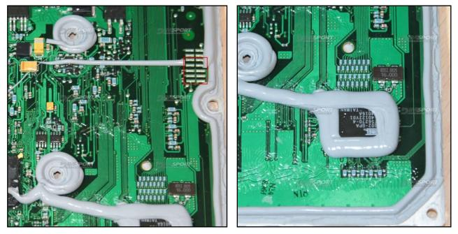
In order to perform the BDM reading it is necessary to make a little bridge on the quartz as shown in the following picture. Remove the bridge from the quartz at the end of the procedure or before restoring the ECU on the vehicle.
