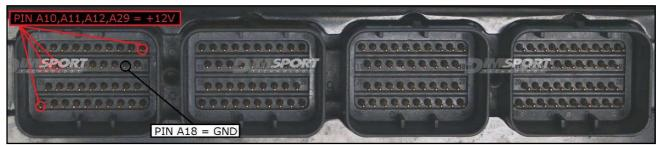
To pin A10,A11,A12,A29 it is possible to connect RED and ORANGE wires, they both are 12V.  ${f J-TAG}$  FREE WIRING CONNECTION
