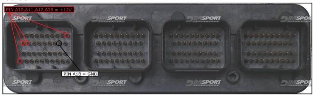
To pin A10,A11,A12,A29 it is possible to connect RED and ORANGE wires, they both are 12V. **J-TAG FREE WIRING CONNECTION**
