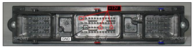
To the power feeding pins (+12V) you can connect both wires red (VECU) and orange VKEY) of the F32GN037C cable, they both have 12V signal.
