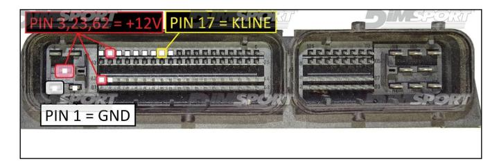
To the power feeding pins 3,23,62 (+12V) you can connect both wires red (VECU) and orange (VKEY) of the F32GN037C/D cable, they both have 12V signal.
