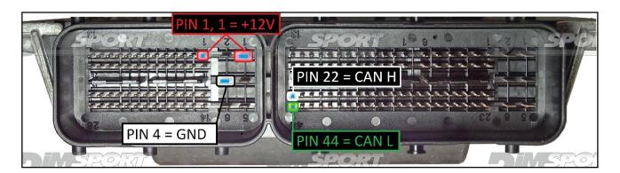
WARNING: due to the relevant power absorbed by the ECU at the beginning of the communication we suggest to feed the ECU with an external power supply or a car battery. Connect the power cable F32GN003 to the Trasdata and then to the power source.
