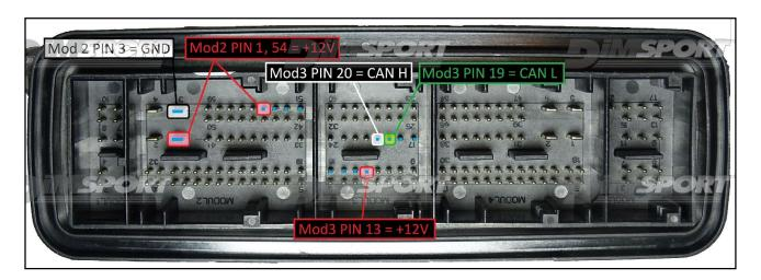
To the power feeding pins 1,54,13 (+12V) you can connect both wires red (VECU) and orange VKEY) of the F32GN037C cable, they both have 12V signal.
