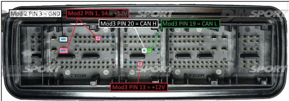
To the power feeding pins 1,54,13 (+12V) you can connect both wires red (VECU) and orange VKEY) of the F32GN037C cable, they both have 12V signal.
