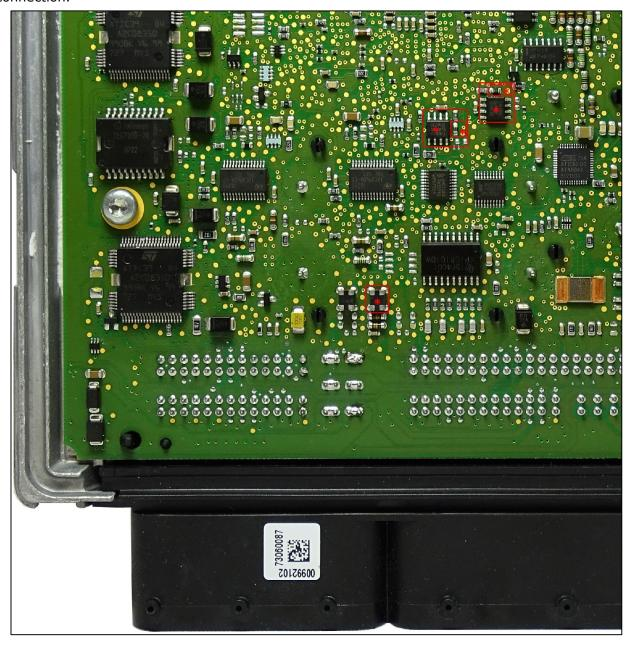
IF on some ECU some components are missing it is necessary to perform the little bridges LINK1 & LINK2 and move the chip 1 & the resistor 2 as displayed in the following pictures. At the end of the operations, before placing back the ECU into the car, it is mandatory to place in their original position the 2 components (chip & resistor) and remove the little bridges LINK1 & LINK2.
