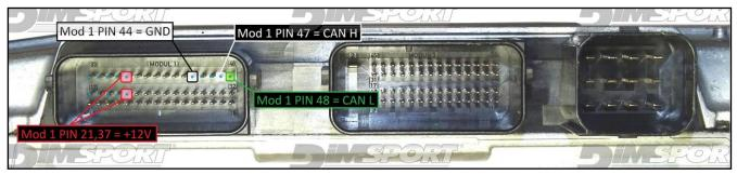
WARNING: due to the relevant power absorbed by the ECU at the beginning of the communication we suggest to feed the ECU with an external power supply or a car battery. Connect the power cable F32GN003 to the Trasdata and then to the power source.
