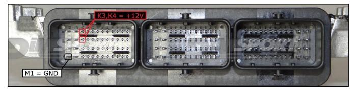
To the 2 power feeding pins K3 and K4 you can connect both wires red and orange, they both have 12 Volt signal.
