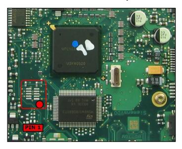
Connect the adapter F34NTA06 as shown in the picture.
