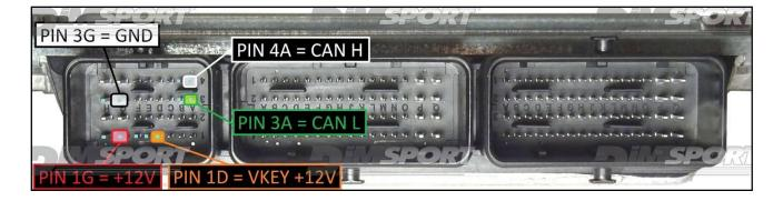
WARNING: due to the relevant power absorbed by the ECU at the beginning of the communication we suggest to feed the ECU with an external power supply or a car battery. Connect the power cable F32GN003 to the Trasdata and then to the power source. The ECU must be powered through the Trasdata using the F32GN037C/D cable
