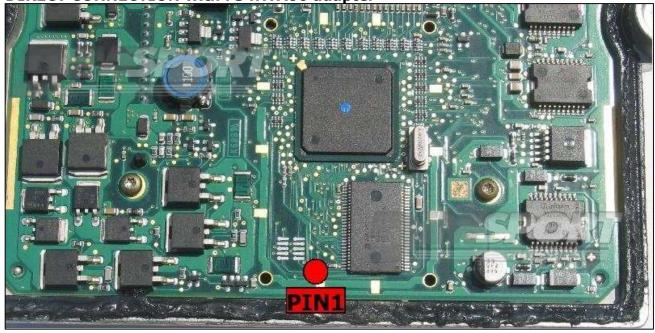
Connect the adapter F34NTA06 as shown in the picture here below.
