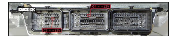
To the power feeding (+12V) C3/G4 pins you can connect both wires red (VECU) and orange (VKEY), they both have 12 Volt signal.
