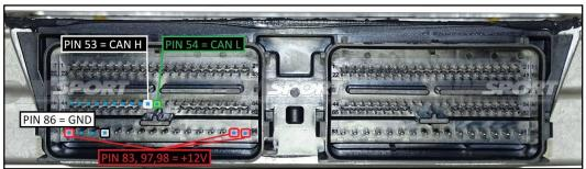
To the power feeding pins 83,97,98 (+24V) you can connect both wires red (VECU) and orange (VKEY) of the F32GN037C cable.
