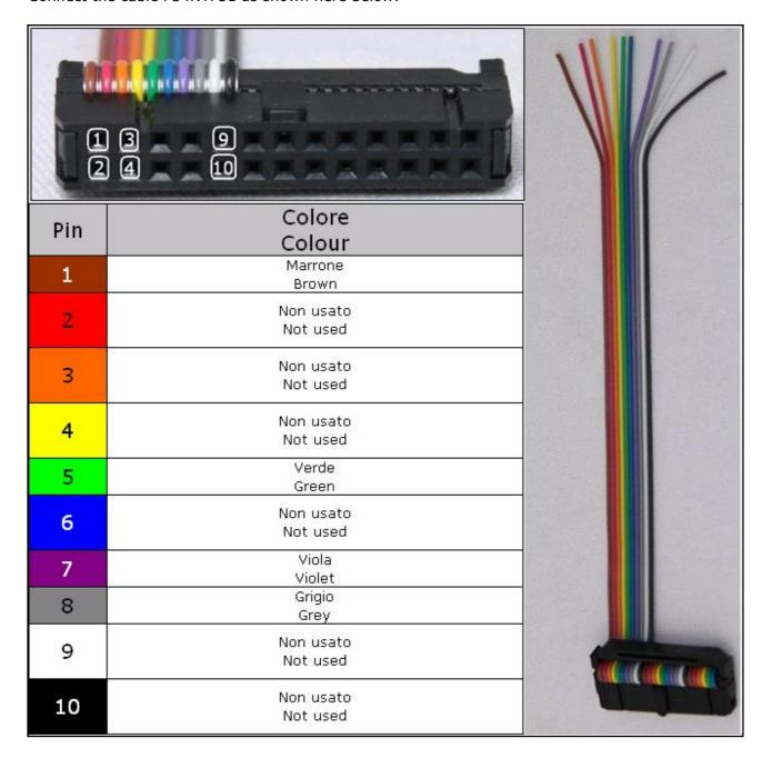
Connect the wires avoiding any short-circuits between the pads
