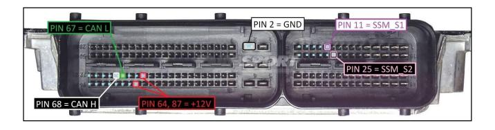
After the correct reading of the password you can open the ECU and perform the connections for the BOOT mode.
