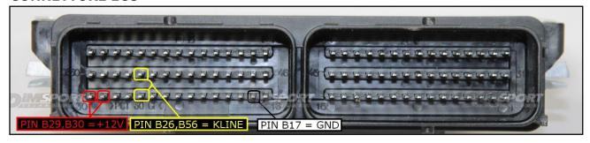
**Warning:** for a correct communication it is necessary to connect the KLINE (yellow wire) to both pins B26 (L Line) and to B56 (K Line).
