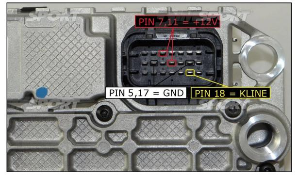
**WARNING:** in order to read the backup file (.BAK) or the microprocessor file it is NOT necessary to open the ECU. The ECU opening is required ONLY for the backup file (.BAK) or eeprom writing procedure.
