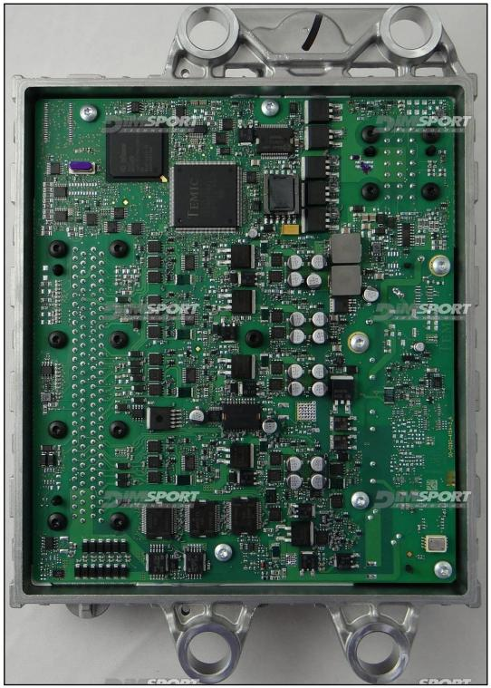
Look for the correct eeprom chip, desolder the pin n.3 of the eeprom, detach it from the board raising up a little bit the pin. Connect the pin 3 directly with the pin n.8. At the end of the writing procedure disconnect the LINK and solder back the pin 3 to the board.
