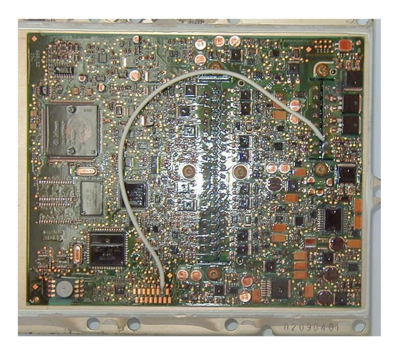
If the Wire wants to be left and close the ecu, use a silicon cable to the resistant to the high temperatures at least up to  $100 \, \text{C}^{\circ}$ .
