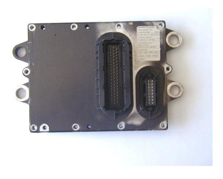
Get off the ecu from the truck, unscrew the screws , and lift the cover very slowly without damaging it.
