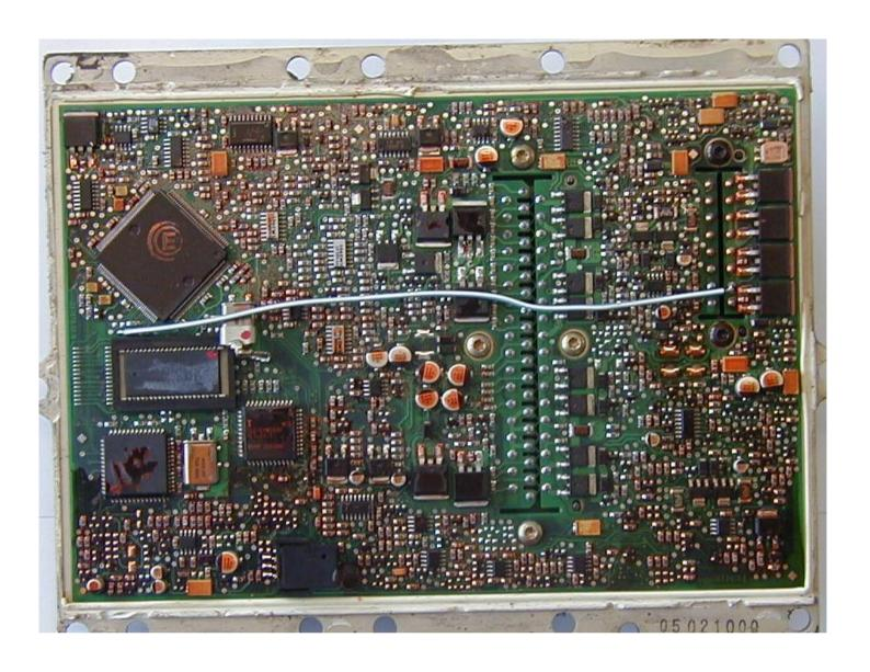
Connection from the pin 7 with 29F200 TSOP.
