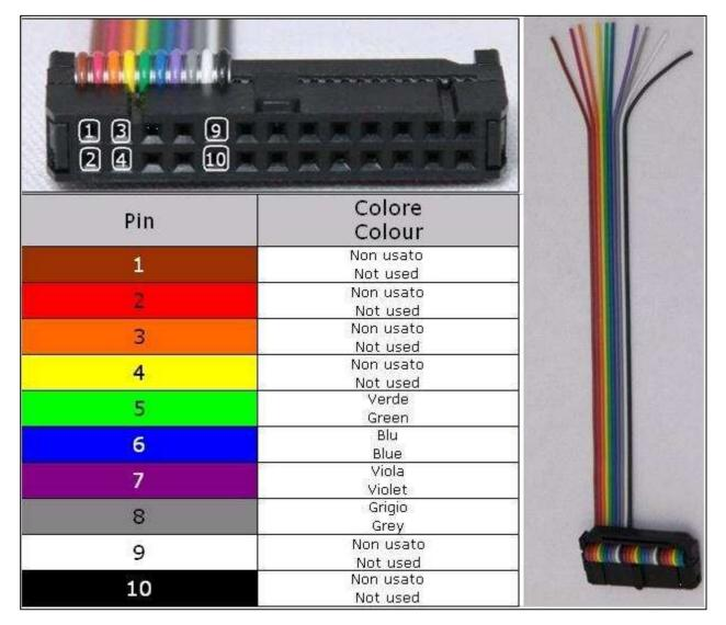
The pin 5 (green) and pin 6 (blue) are placed on the upper side of the ECU, the pin 7 (violet) and 8 (grey) are placed on the lower side of the ECU.
