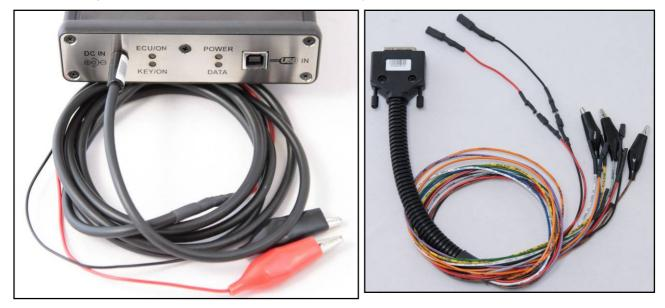
To power the ECU connect the red wire (+ 12V) and black wire (GND) of F32GN037C/D wiring to the ECU pin connector shown here below:
